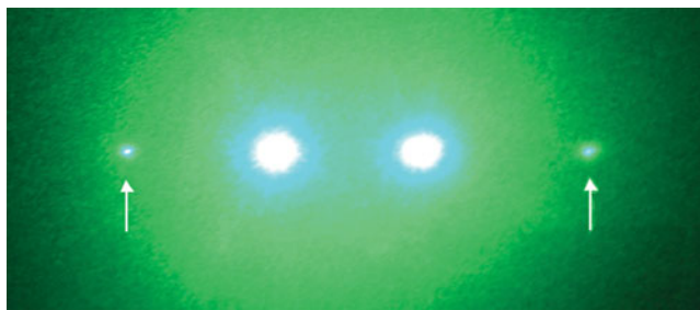
Figure 4a. The reconstructed photothermoplastic hologram of a planar wavefront image recorded in the composite sample with a free film surface (glass substrate – ITO – composite film) based on OGC doped with 10 mass % DPPH ( L \sim 1 \mu\text{m} ) under sample illumination by green semiconductor laser ( I = 15 \text{ mW} , t_{\text{exposure}} = 5 \text{ s} ) irradiation. Hologram was recorded at a 1:1 intensity ratio of the reference to the object beam. The spatial frequency of hologram recording was \sim 800 \text{ mm}^{-1} . The diffraction efficiency value \eta was \sim 0,25\% (the corresponding diffraction orders are shown by vertical arrows).
